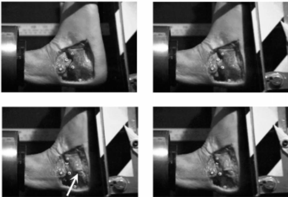
Figure 3: (upper left) dorsiflexed specimen before impact, (upper right) initial contact, (lower left) with loss of joint space crack forms on plantar surface of calcaneus (arrow), (lower left) calcaneus fractured.
