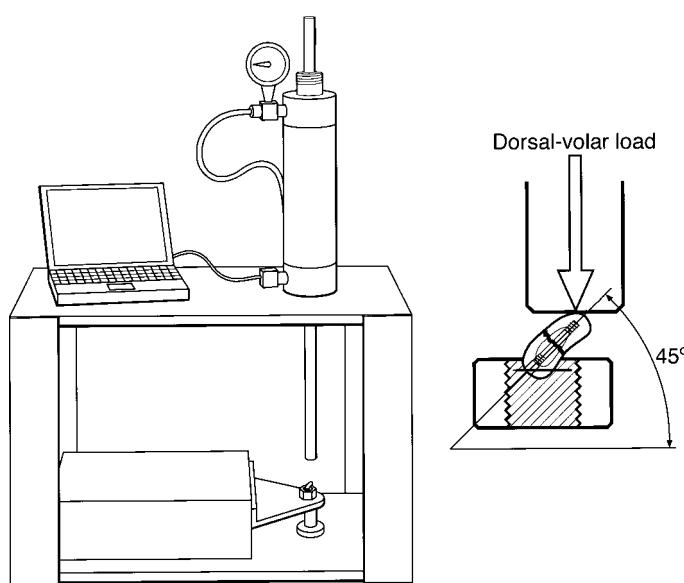
Figure 3: Schematic depicting the potted scaphoid specimen and testing apparatus for delivery of dorsal-to-volar cantilever bending load.
