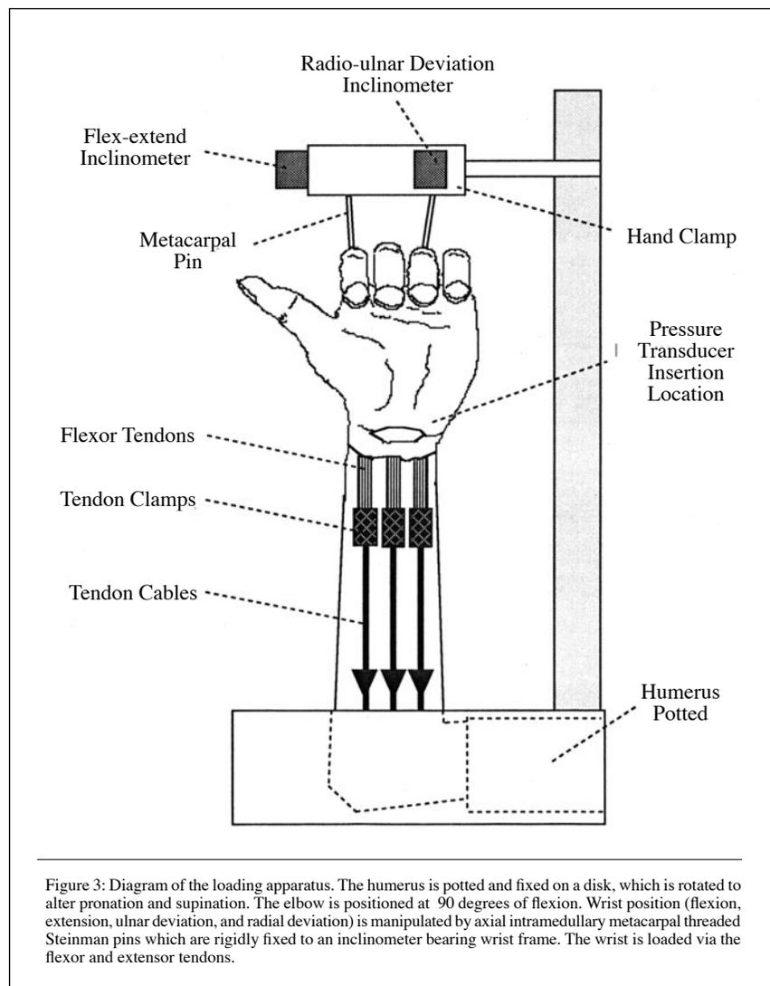
Figure 3: Diagram of the loading apparatus. The humerus is potted and fixed on a disk, which is rotated to alter pronation and supination. The elbow is positioned at 90 degrees of flexion. Wrist position (flexion, extension, ulnar deviation, and radial deviation) is manipulated by axial intramedullary metacarpal threaded Steinman pins which are rigidly fixed to an inclinometer bearing wrist frame. The wrist is loaded via the flexor and extensor tendons.
