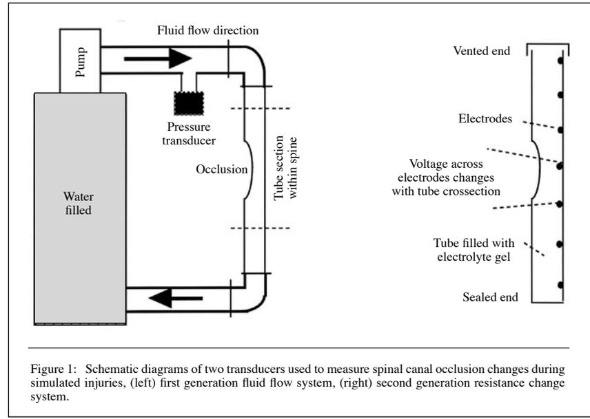
Figure 1: Schematic diagrams of two transducers used to measure spinal canal occlusion changes during simulated injuries, (left) first generation fluid flow system, (right) second generation resistance change system.
