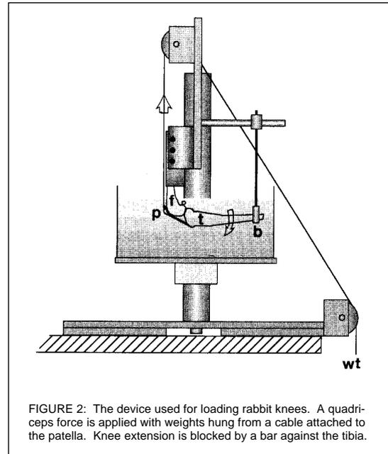
FIGURE 2: The device used for loading rabbit knees. A quadriceps force is applied with weights hung from a cable attached to the patella. Knee extension is blocked by a bar against the tibia.
