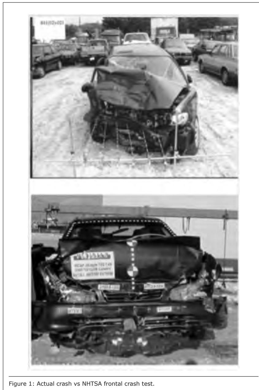
Figure 1: Actual crash vs NHTSA frontal crash test.
